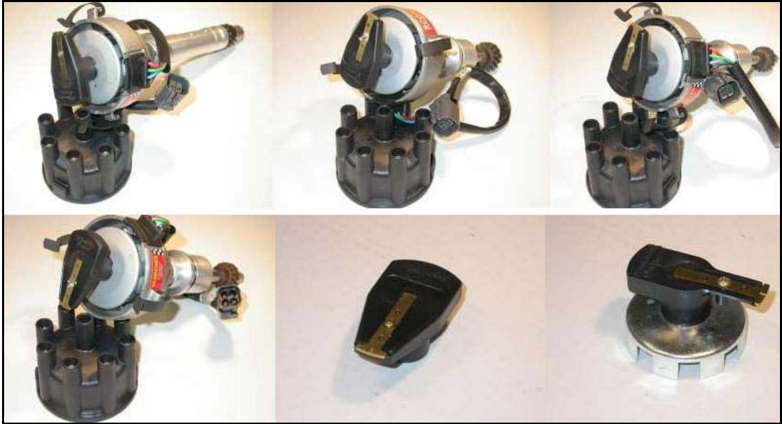
Row 1: Chev small block, Cleveland, Windsor 289, Row 2: Windsor 351, Rotor button, Rotor button and disk
