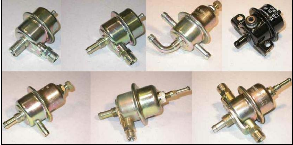
Row 1: 2.5bar screw, 2.5bar single, 3bar dual, 3bar O ring, Row 2: 3bar single, 2-4bar adjustable, 2-5bar adjustable
